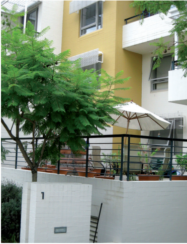
Private balconies and appropriate building setbacks promote casual surveillance and opportunities for outdoor living.
